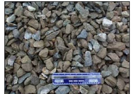
Figure 6. No. 4 crushed limestone.
